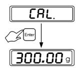
Please use , , , , key to key in the mass values which you are going to calibrate, then press key to confirm the value. When the display is flashing and showing the weight values, put the mass on scale. While scale is stable, the scale will return back to weighing mode. The calibration procedure is finished.
